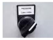
DUAL PRESSURE SETTING Enables the machine to change from high pressure to low pressure to bale both cardboard and plastic.
