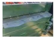
AGCRESSIVE HEAD RAM This consists of aggressive blades designed in a "V" shape to improve shearing when baling bulky or rigid materials.
