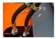
ANTI-WHIP PROTECTION Mechanical restraint used to prevent uncontrolled hose movement in the event of hose or coupling failure.
