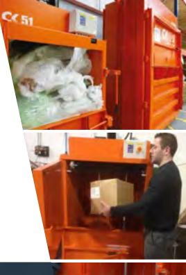
Waste Baling Machine's standard vertical balers range is suitable for a wide variety of applications including baling plastic and cardboard. These balers produce bales of cardboard from 50kg up to 500kg.
